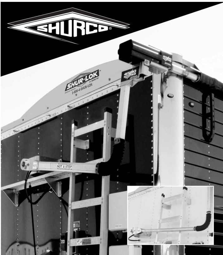
Above: The 4500 Series HD with its super-strong, heavy-duty torsion arms.
