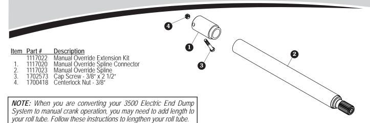
STEP 1: After Gate Flex™ and flex arm have been removed from rear of trailer, place manual override spline connector over splined shaft on roll tube.
