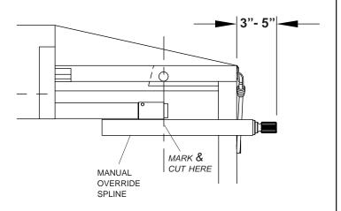
STEP 3: Remove manual override spline connector from roll tube and weld connector to manual override spline. Grind
