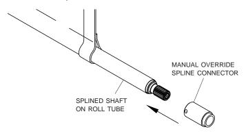
STEP 2: Align manual override spline with roll tube on side of trailer so end of spline extends 3" to 5" past rear of trailer. Mark and cut manual override spline as shown.
