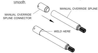
STEP 4: Install manual override extension weldment over splined shaft on roll tube. Secure with 3/8" x 2 1/2" cap screw and 3/8" centerlock nut (from Gate Flex™).
