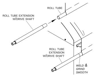
**NOTE:** To prevent rust, paint all exposed metal, such as weld seams and/or metal exposed by grinding or cutting, with corrosion-resistant paint.
