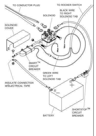
**STEP 7:** Mount rocker switch in cab in convenient location on dash panel or door jamb. Crimp female quick disconnects and connect to rocker switch as shown.
