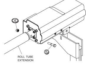
**STEP 5:** Install crank arm assembly as shown in Shur-Lok<sup>®</sup> owner's manual. Manual may be viewed at http:// www.shurco.com. You may need optional manual override extension kit (P/N 1117022).
