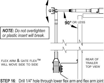
STEP 16: Drill 1/4" hole through lower flex arm and flex arm joint as shown. Install 1/4" x 1-3/4" spring pin into drilled hole.
