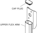
STEP 3: Thread end fitting onto end of flex arm joint assembly. Tighten so end fitting is parallel to existing end fitting.
