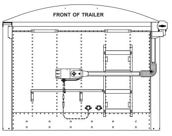
**NOTE:** Wire lengths are predetermined. Before installing SMARTwire<sup>™</sup> components, review and confirm wire routing so wires reach components with ample room for connection.
