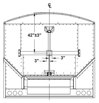
**STEP 2:** Place mounting beam on trailer as shown. Using beam as guide, determine mounting hole locations.
