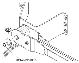
**STEP 5:** Choose appropriate pilot hole on pivot bracket to route 6-ga. wire from flex arm through trailer skin. Fasten wire clip to pilot hole with 1/4" x 3/4" self-drilling screw.
