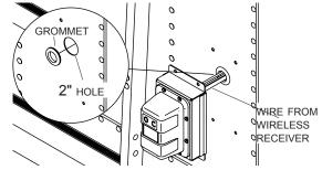
STEP 4: Align holes on wireless receiver with holes on trailer. Fasten receiver to trailer with 5/16" x 7/8" cap screws
