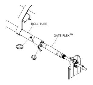
**STEP 2:** Carefully slide Gate Flex<sup>™</sup> off roll tube. Flex arm will be under tension and have some downward force.
