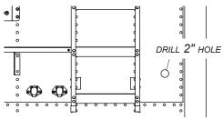
**STEP 2:** Align holes in wireless receiver over 2" hole in trailer as shown below. Using holes on flanges on receiver as guide, mark and drill four 5/16" holes as shown.
