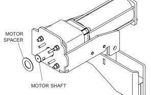
STEP 6B: Slide roll tube extension over motor shaft. Fasten with 3/8" x 2" cap screws ஹ and lock nuts ୠ. Finger tighten only.
