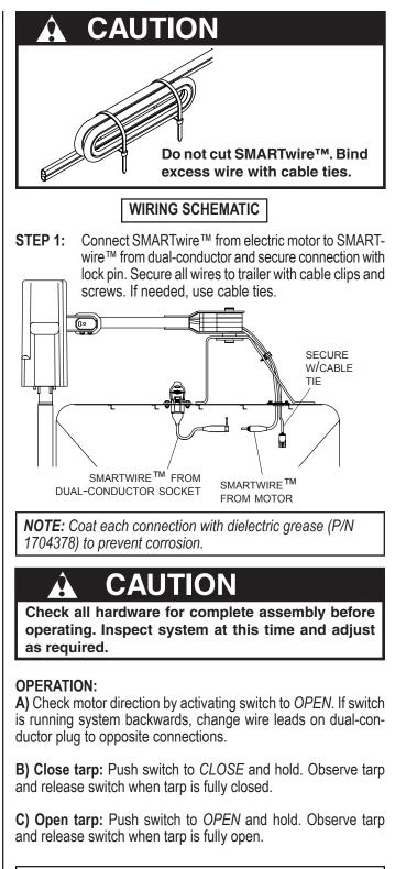
**NOTE:** Release switch at end of cycle or modified-reset circuit breaker will trip. After breaker resets, switch will activate motor again. To reduce unnecessary strain on tarp components, release switch at end of each cycle.
