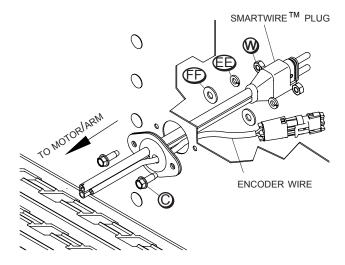
**STEP 9:** Remove cable tie from front arm/motor assembly before operating system.
