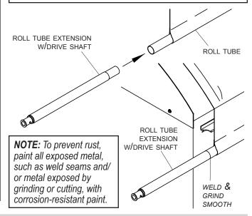
**STEP 10**: Slide roll tube/roll tube extension weldment back into position and align upper flex arm on front of trailer. Follow step 11 to install motor, positioning motor as shown below. Make sure torsion springs load when tarp opens.
