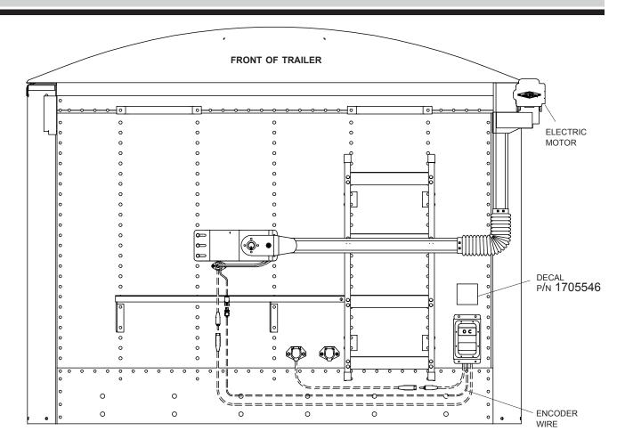
**NOTE:** Wire lengths are predetermined. Before installing SMARTwire<sup>™</sup> components, review and confirm wire routing so wires reach components with ample room for connection.
