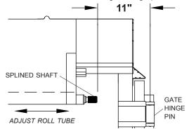
STEP 2: Slide roll tube bearing pack completely over splined shaft on roll tube. Fasten with 3/8" x 2-1/2" cap screw
