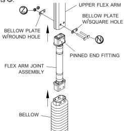
STEP 5: Align holes in end fittings and bellow plates with holes in lower flex arm assembly as shown. Temporarily install 5/16" x 2-1/2" carriage bolts 𝔅 and lock nuts 𝔅.
