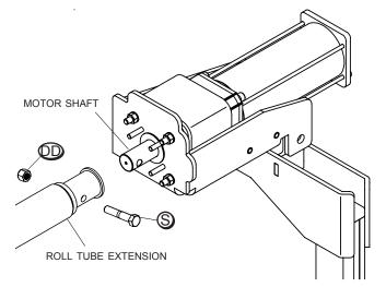
**STEP 7:** Hold flex arm with motor and roll tube extension in vertical plane to trailer and 90° to roll tube. Mark and cut roll tube at location shown.
