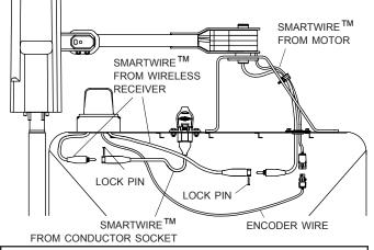
**NOTE:** Coat each connection with dielectric grease (P/N 1704378) to prevent corrosion.
