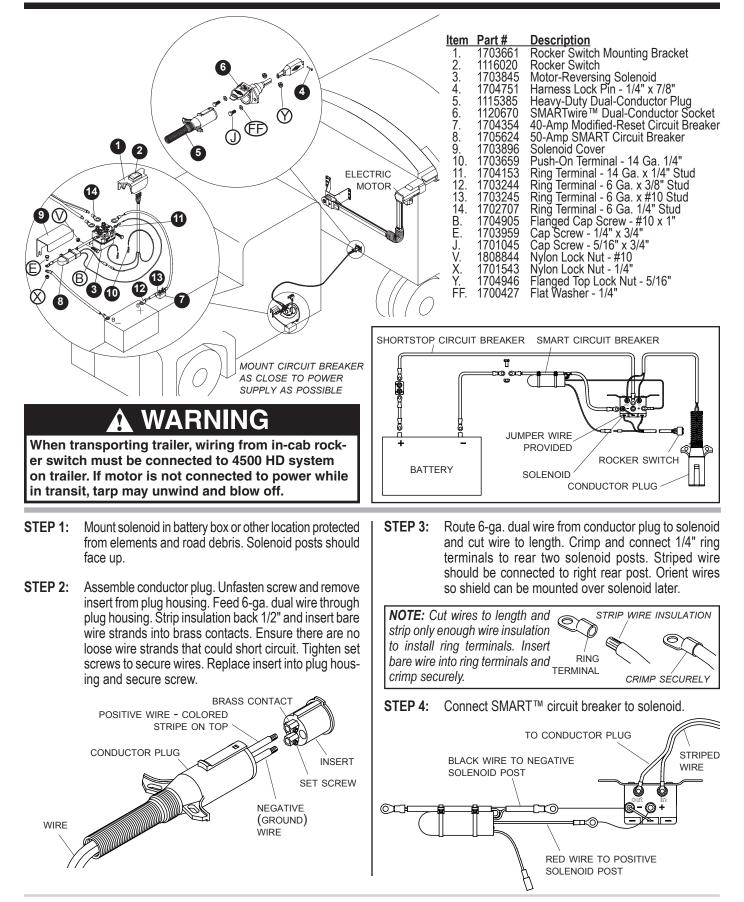
**STEP 5:** Connect SMART<sup>™</sup> breaker to battery. Make jumper out of black 6-ga. wire (no stripe). Connect one end to battery negative post and bolt other ring terminal to SMART<sup>™</sup> breaker. Insulate bolted connection with electrical tape.
