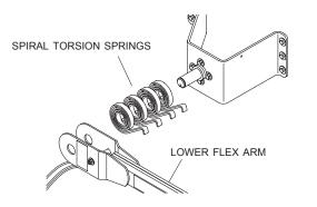
STEP 4: Secure with 1-1/4" flat washer 3 and retaining ring.
