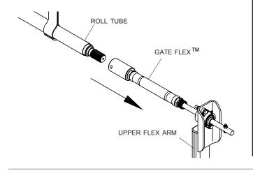
**STEP 3:** Remove retaining ring on rear flex arm. Carefully slide arm off pivot pin.
