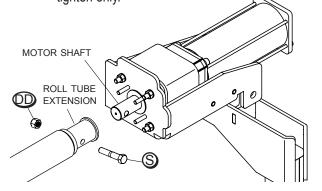
**STEP 7:** Hold flex arm with motor and roll tube extension in vertical plane to trailer and 90° to roll tube. Mark and cut roll tube at location shown.
