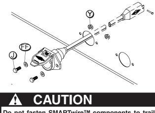
Do not fasten SMARTwire™ components to trailer through hopper walls.
