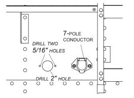
**STEP 2:** Align socket over 2" hole. Using holes in flanges on socket as guide, mark and drill two 5/16" holes.
