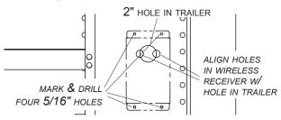
**STEP 3:** Install grommet into 2" hole. Insert wire from wireless receiver through grommet.
