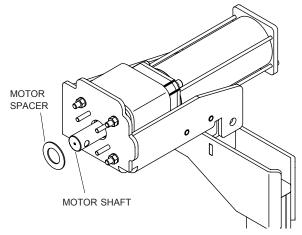
STEP 6B: Slide roll tube extension over motor shaft. Fasten with 3/8" x 2" cap screws 𝔅 and lock nuts 𝔅. Finger tighten only.
