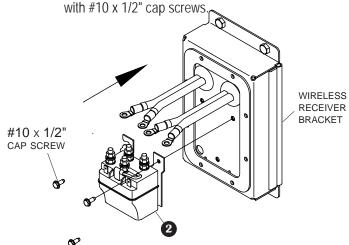
STEP 4: Remove receiver bracket from trailer and install encoder wire **9** through drilled hole from back side of bracket. Feed one connector at a time through drilled hole.
