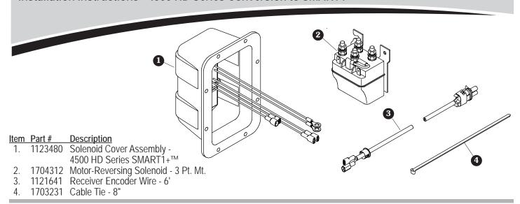
STEP 1: Disconnect power to receiver. Remove existing gray cover and RF solenoid from receiver bracket.
