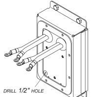
STEP 3: Install solenoid **②** onto wireless receiver bracket. Fasten with #10 x 1/2" can scrows
