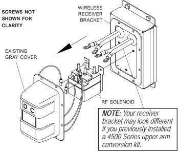
STEP 2: Using pilot hole in receiver bracket as guide, drill 1/2" hole in bracket.
