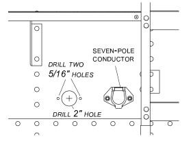
STEP 2: Align socket over 2" hole. Using holes in flanges on socket as a guide, mark and drill two 5/16" holes.
