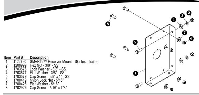
**NOTE:** Receiver mount bracket is designed to support wireless receiver where suitable flat, wide, vertical mounting surface on trailer does not exist.
