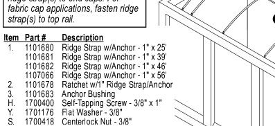
STEP 1: Mark hole locations at center of front and rear caps (mark top rails for fabric caps).
