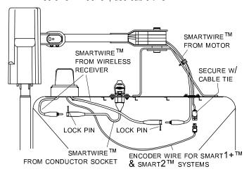
**NOTE:** Coat each connection with dielectric grease (P/N 1704378) to prevent corrosion.
