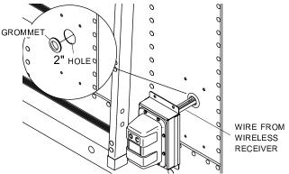
STEP 4: Align holes on wireless receiver with holes on trailer. Fasten receiver to trailer with 5/16" x 7/8" cap screws, lock washers and nuts. Adhere warning decal P/N 1705546 above receiver in location shown.
