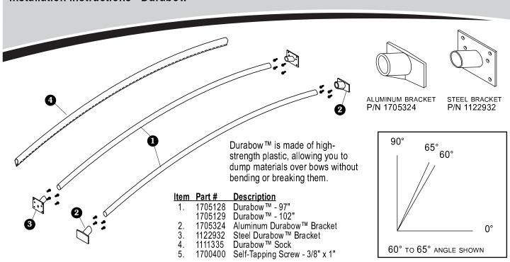
STEP 1: Equally space bow brackets on either side of trailer.
