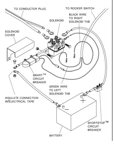
STEP 7: Mount rocker switch in cab in convenient location on dash panel or door jamb. Crimp female quick disconnects and connect to rocker switch as shown.
