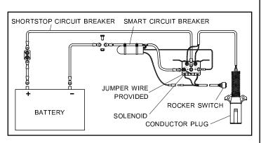
STEP 1: Mount solenoid in battery box or other location protected from elements and road debris. Solenoid posts should face up.
