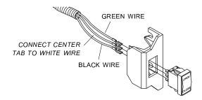
**STEP 8:** Route 14-ga. 3-conductor cable between rocker switch and solenoid.
